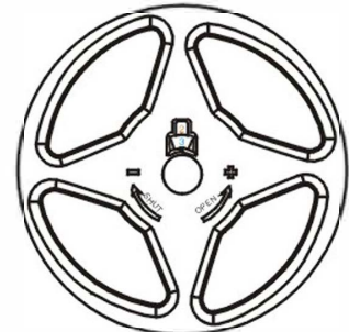
Fig. 2 The Valve Is Set At 2.3 Turn
