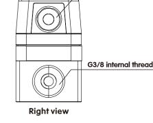
Note: The example of G3/8 femalel thread and aviation plug connector outlet is used as an illustration.
