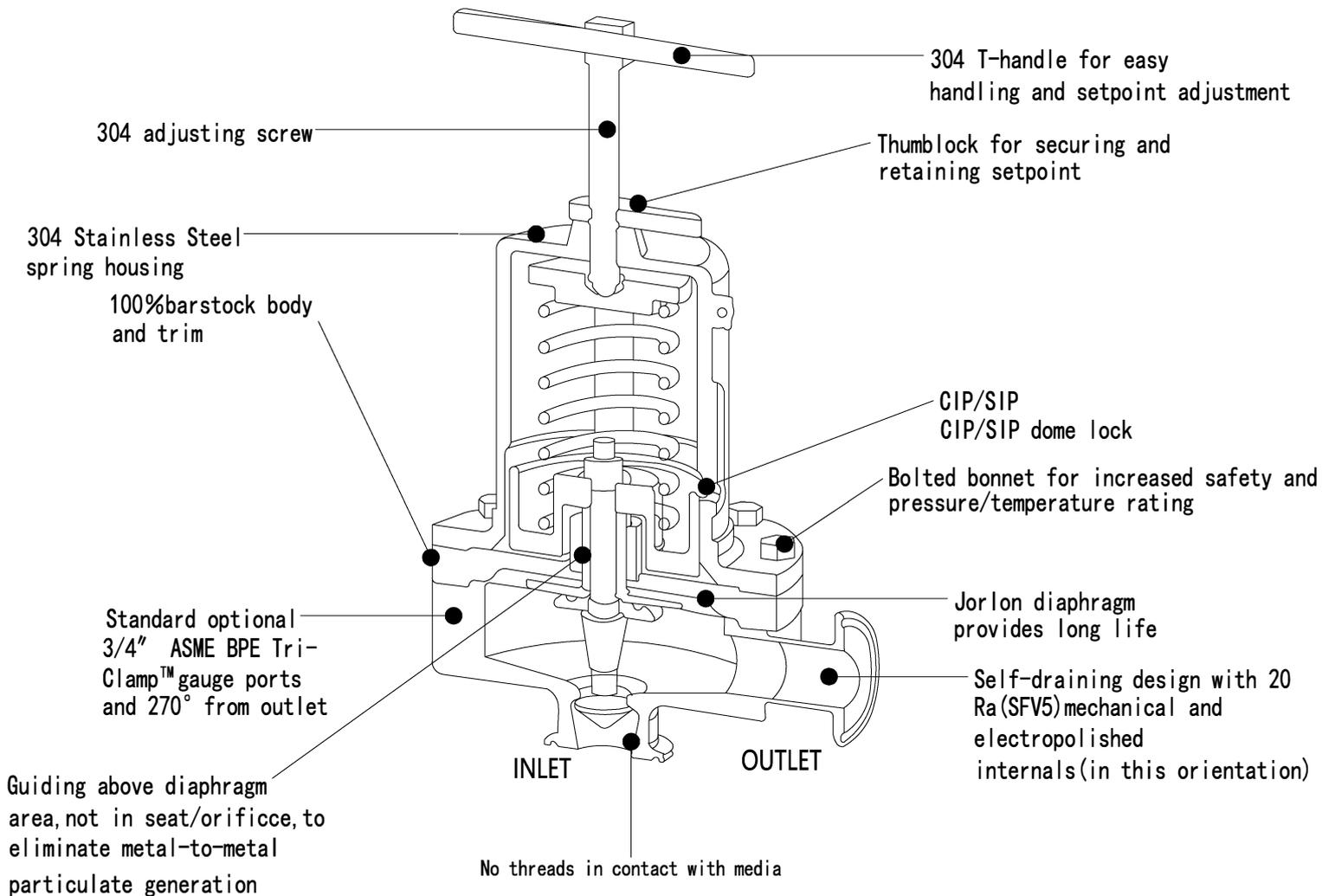
Body Pressure Temperature Rating: (dependent upon construction)
