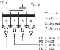
When install several proximity sensor near by, it may cause malfunction due to mutual interference. Therefore please use Differential frequency for the application.
